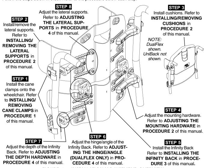
FIGURE 1 - INSTALLATION/ADJUSTMENT OVERVIEW
